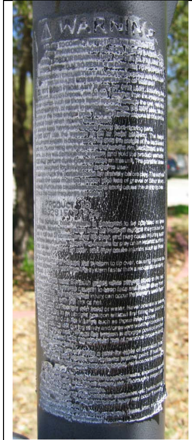
Figure 5. The warning on this basketball stand has become worn due and can no longer be read or understood.
